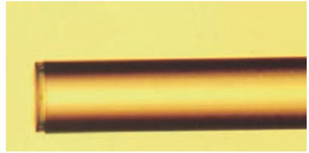
Fig. 5: Miniature all silica pressure sensor.
