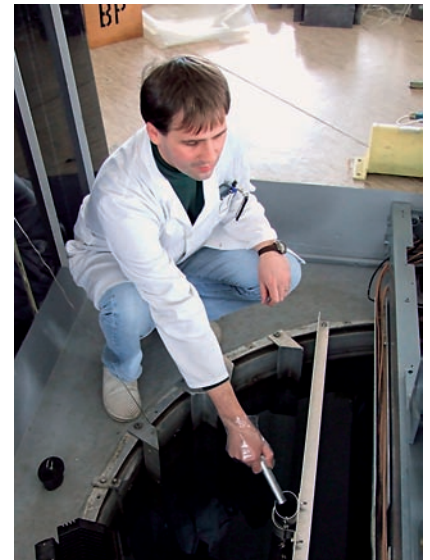
Dr Tomaž Žagar introducing a ceramic sample into the irradiation channel in the TRIGA Mark II.
