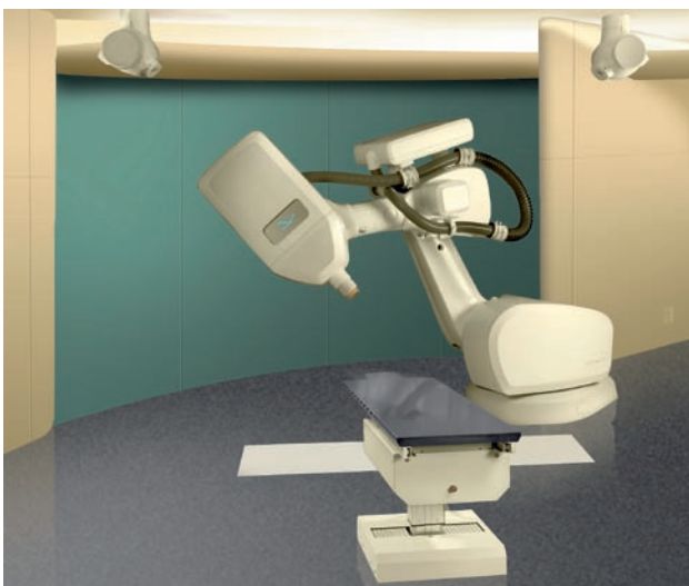
CyberKnife incorporating a miniature linac waveguide mounted on an industrial robotic arm for dose delivery and two orthogonal planar x-ray imaging systems for determination of target location. (Courtesy of Accuray, Inc.)
